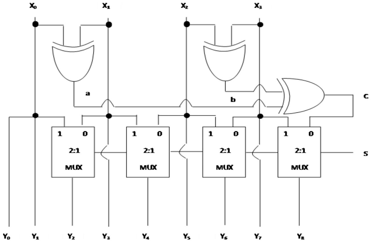
Figure 3: Encoder Circuit Based on Error Correcting Coding Method
