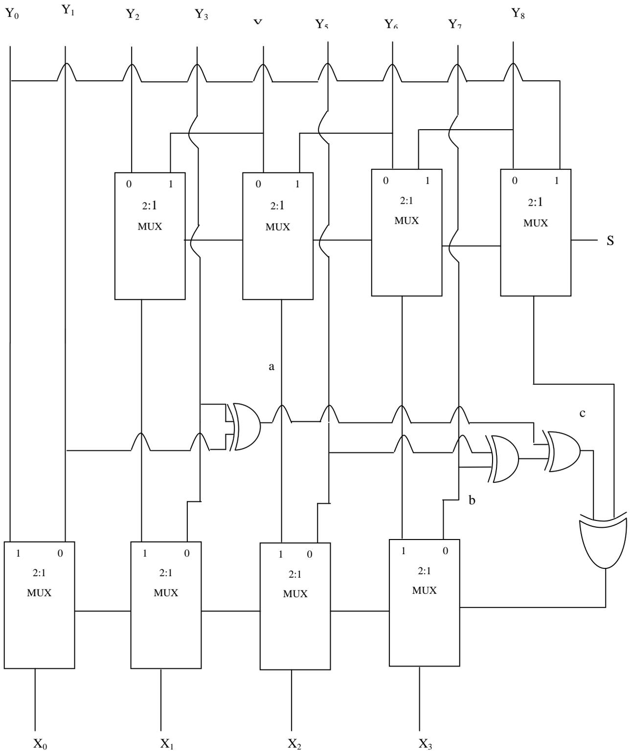
**Figure 4: Decoder Circuit Based on Error Correcting Coding Method**
