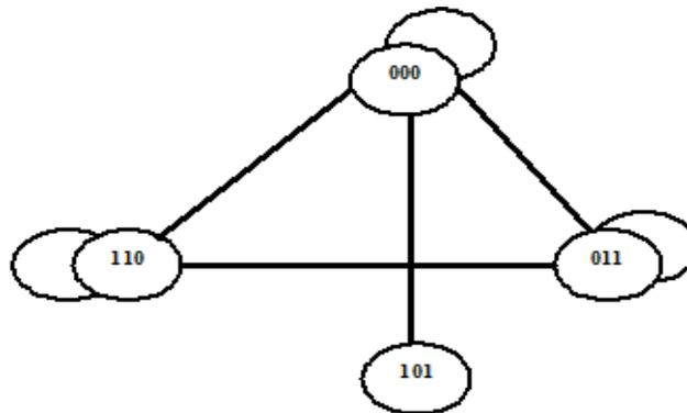
Figure 1: Graphical Representation of Single Error Detecting 3- Bit Self Shielding Codes
