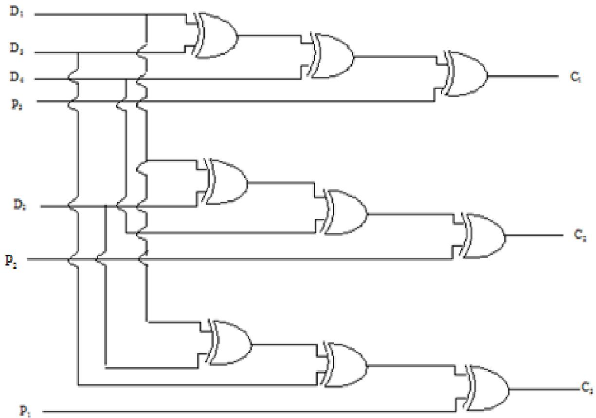
Figure 2: Parity Check Circuit
